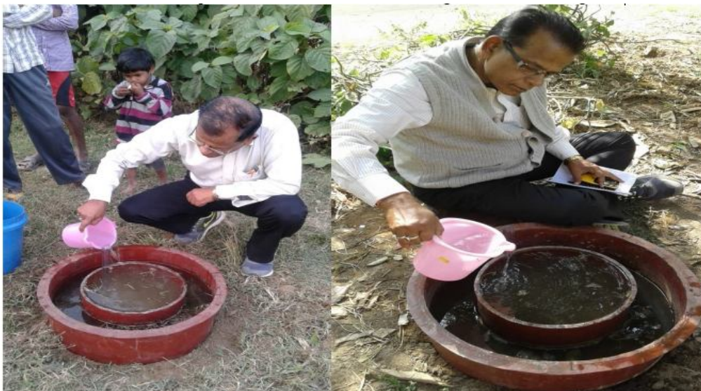
Figure 3: Installing and reading off the double ring infiltrometer.
