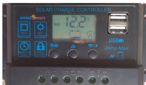
Fig. 2: PWM Solar Charge Controller
