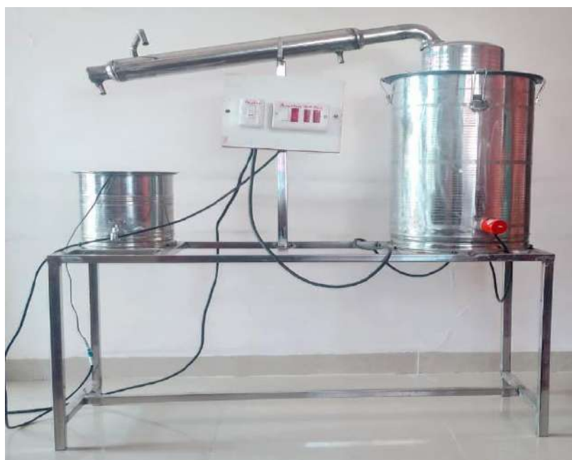
Fig. 1 Experimental Setup of Steam Distillation Unit
