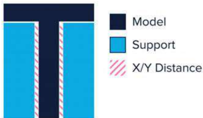
Fig. 4 Showing part orientation and support material. (Image Source: ALL3DP)
