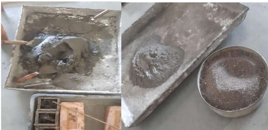
Fig.4 Mixing of Mortar
