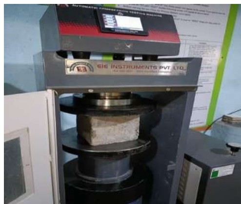
Figure1: Compressive strength test for concrete specimen.
