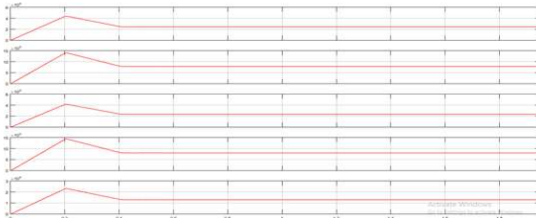
Fig. 6.3 Wavelet spectral energy of multi resolution analysis signals detail D1 to D4 and Approximation A4 signal of three phase current when islanding occurs at generator 1 at 0.2 sec time
