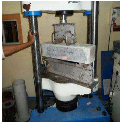
Figure 2: flexural strength testing of concrete Specimen
