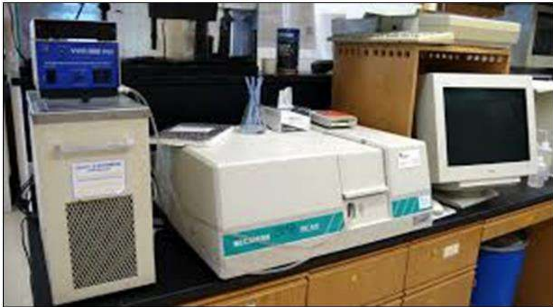
Fig 3(a) Basic design of UV-Vis Spectrophotometer
