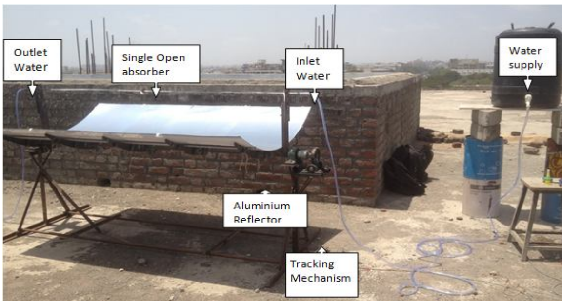
Fig-1: Experimentation set up for open tube absorber mounted parabolic trough
