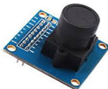
Figure-2.2: OV7670 640×480 VGA CMOS Camera Image Sensor Module
