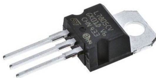
Fig: Voltage Regulator
