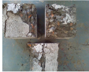
Fig-2: Shows the failure pattern of cube specimens.
