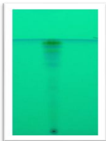
Figure 2 TLC Fingerprinting of Hexane: Ethyl acetate (9.8:0.2) solvent system of Aegle marmelos
