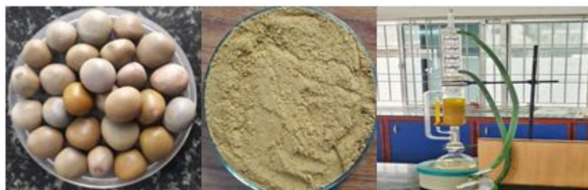
Fig: 3. Extraction of Caesalpinia bonducella seeds with ethanol by Soxhlet apparatus [11].
