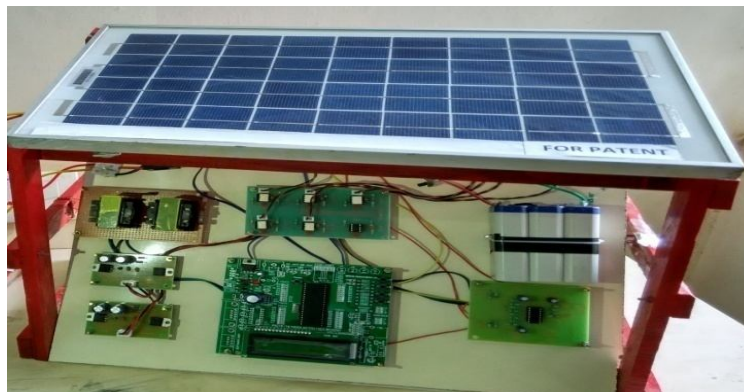
Fig 8. The Prototype with Solar PV Panel
