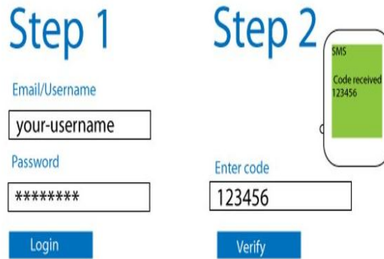
Fig 3.1: Mechanism of Two Step Verification [5] Source
