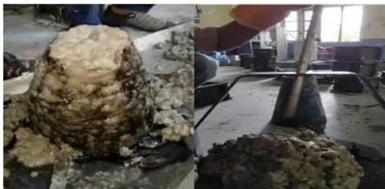
Fig: 1 Slump test results with different liquid binder ratios
