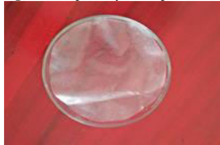
Fig-6 Lab level preliminary output – biodegradable bag- product development
