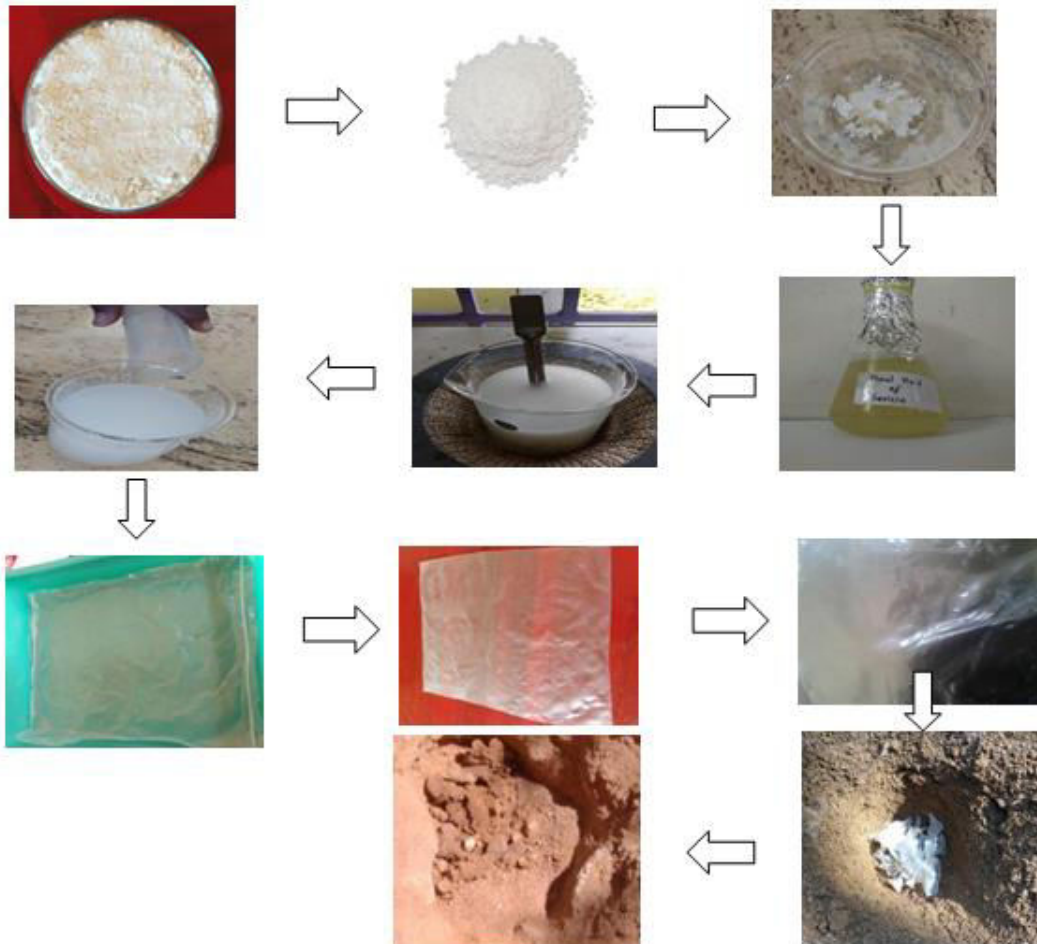
Fig-6 Lab level preliminary output – biodegradable bag- product development
