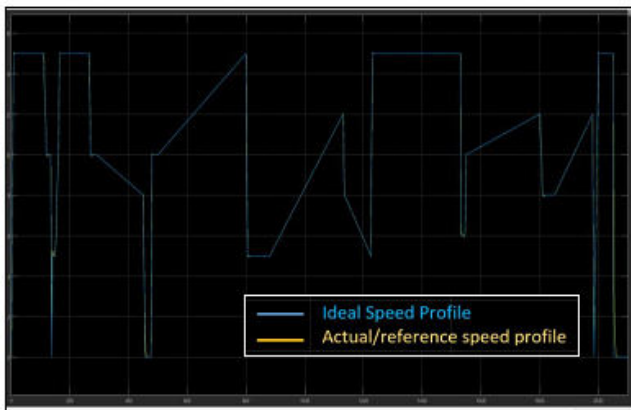
Figure 4. Ideal and actual/reference speed profiles on the Experimentation Drive Cycle. (Speed in KMPH vs Time in seconds.)
