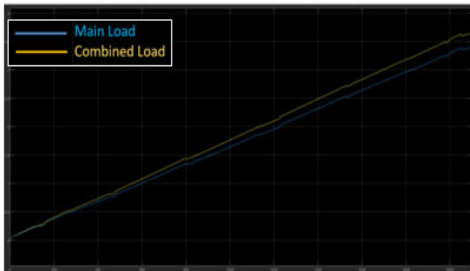
Figure 8. Battery packs energy in KWh vs time in seconds.
